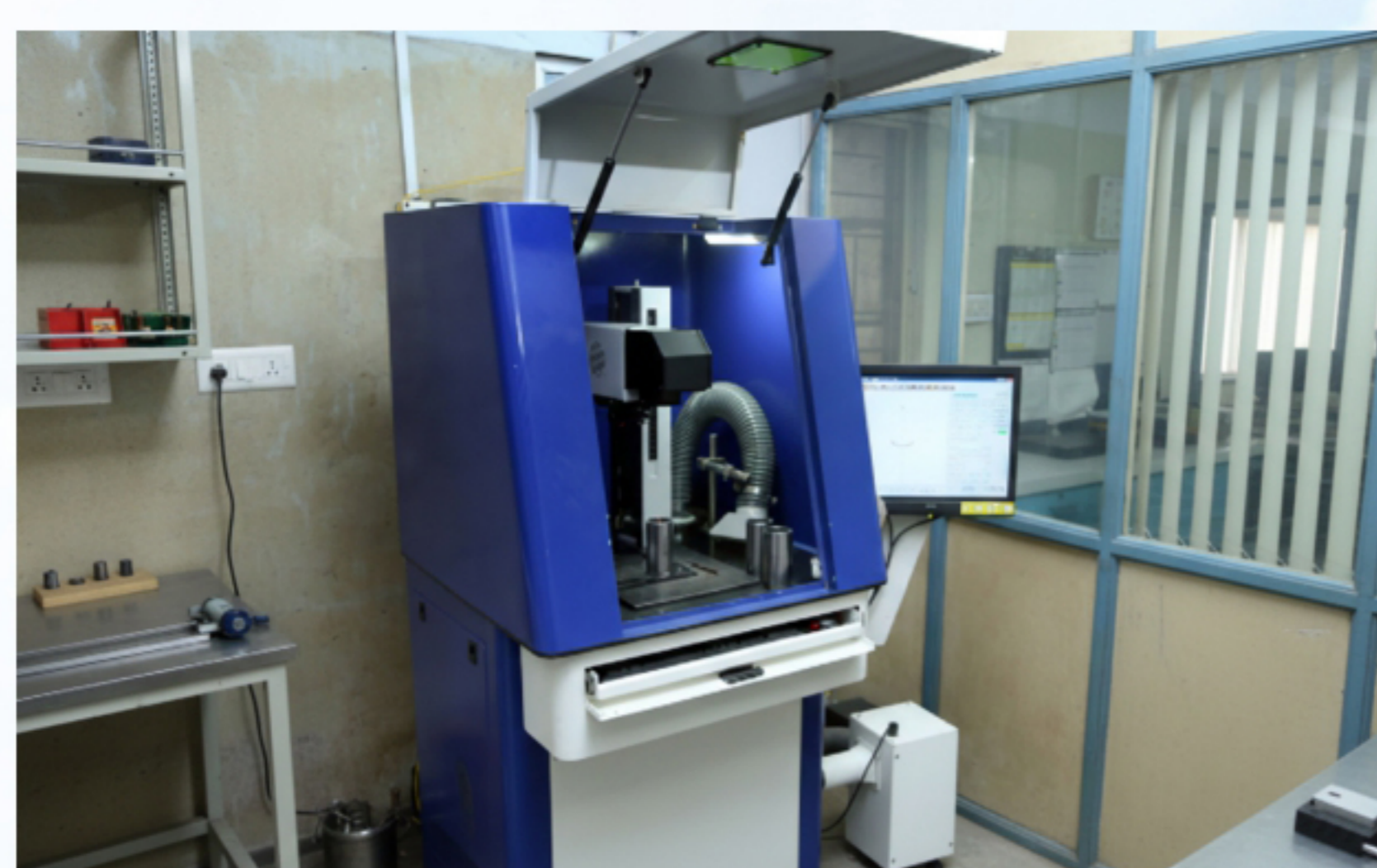
Pressure Leakage test upto 300 BAR
